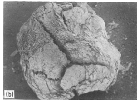
Figure 2 Scanning electron micrograph of the HD powder prior to milling. (a) High magnification picture of flake-like material ( \times 15 ). (b) Formation of flakes from a larger particle ( \times 5.5 ).
