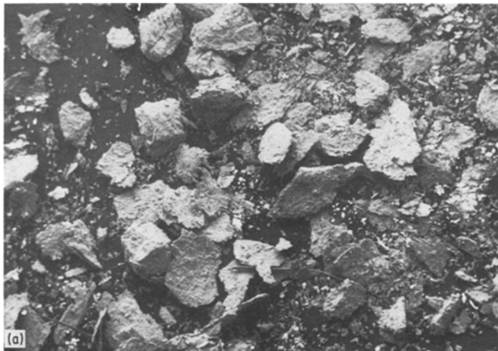
Figure 2 Scanning electron micrograph of the HD powder prior to milling. (a) High magnification picture of flake-like material ( \times 15 ). (b) Formation of flakes from a larger particle ( \times 5.5 ).
